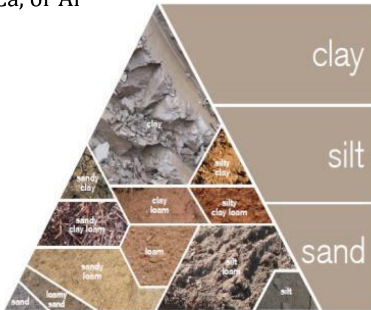
FIGURE 2.2 - SOIL TEXTURE TRIANGLE
